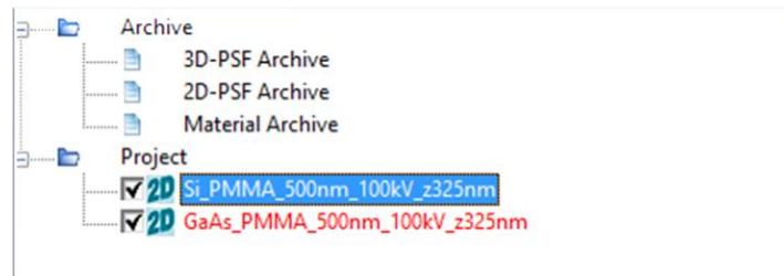
Figure 4. Two PSFs selected in TRACER. The Silicon PSF is highlighted as the base PSF.
