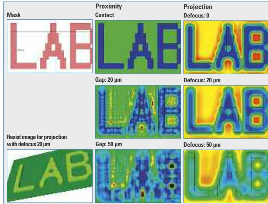
Projection lithography simulation has been a key enabler for IC manufacturing to keep track with market demands and Moore's law. Although 30 years ago the end of optical lithography was predicted for feature sizes < 1μm, optical lithography is currently doing < 30nm today in volume manufacturing. Without lithography simulation and the simulation based resolution enhancement techniques such as OPC, source shaping and source mask optimization these dimensions would never have been possible.
